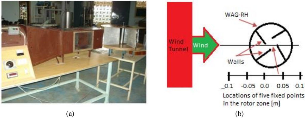
Fig. 3 (a) Experimental setup and (b) experimental layout showing five important locations in the rotor zone in stream-wise direction where measurements were taken.
